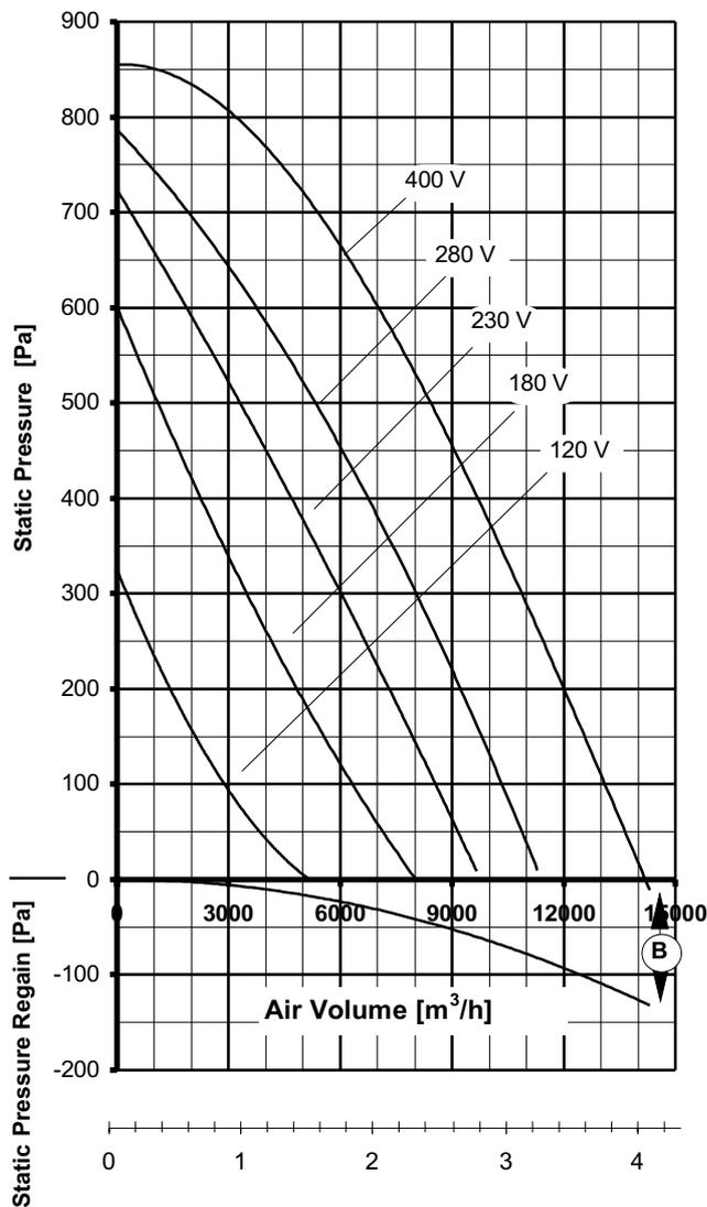
The data for external static pressure take into account all pressure losses due to integration of the fan within unit. Performance based upon free inlet and discharge.
